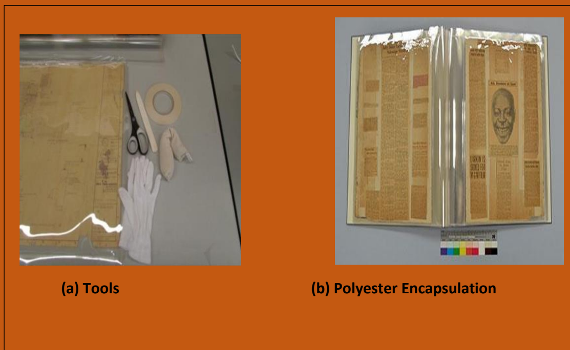
Fig.5: Tools used for Encapsulation: White cotton gloves, polyester encapsulation film, double-sided encapsulating tape, weights, bone folders and scissors.
